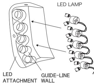
※ Use heat resistant caulking glue to fix the attached LED lamps.
