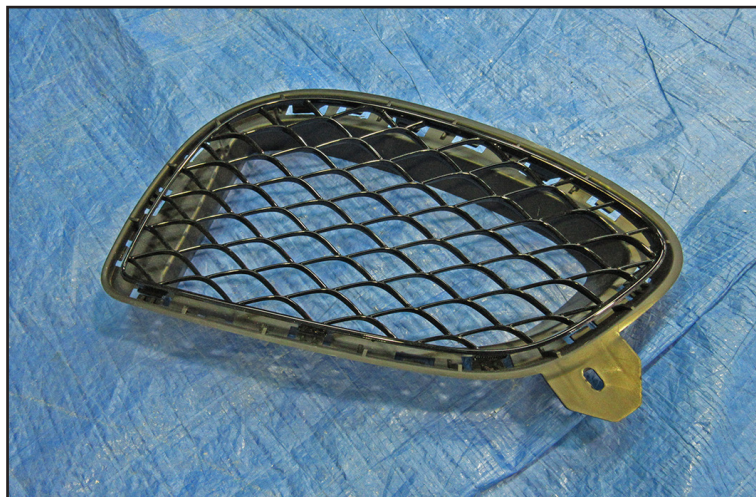
The Above Picture : OEM Side Bumper Duct Mesh Separate the Mesh from the frame.
