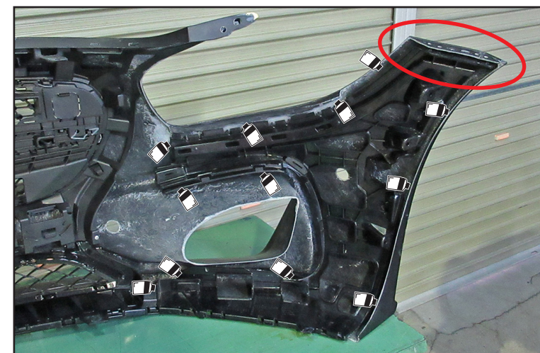
The Above Picture : Side Part of WALD Front Bumper (Inside). Use caulking glue to fix OEM brackets on both side. Red Circled : Fix OEM Side Retainer with the attached rivets.
