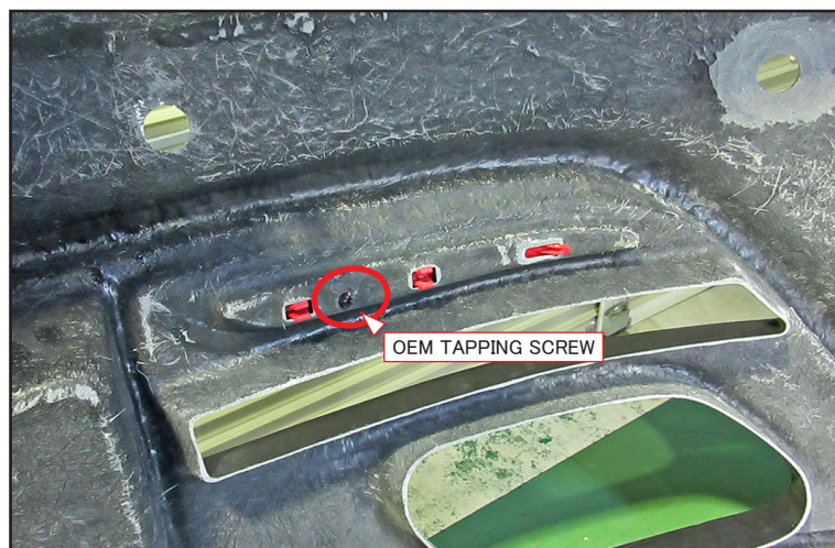
Use OEM tapping screws to fix OEM reflectors in the same way for OEM rear bumper. ※Recommendation : Use caulking glue to fix the nails for prevention of falling.
