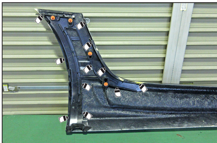
Use caulking glue to fix OEM retainers on WALD Side Steps.
