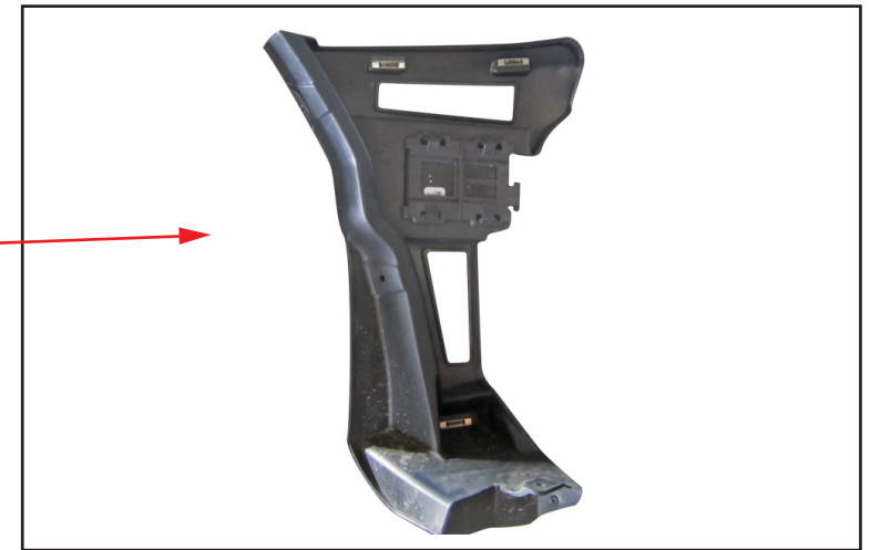
Picture of OEM basement for the sensor. Use the caulking glue to fix them to the same location on WALD Rear Bumper.
