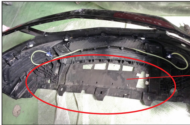
Replace the red circled OEM under cover to WALD Front Bumper.
