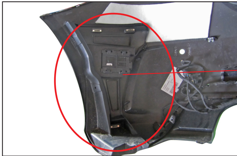
Replace the red-circled OEM sensor units and basements to WALD Rear Bumper.
