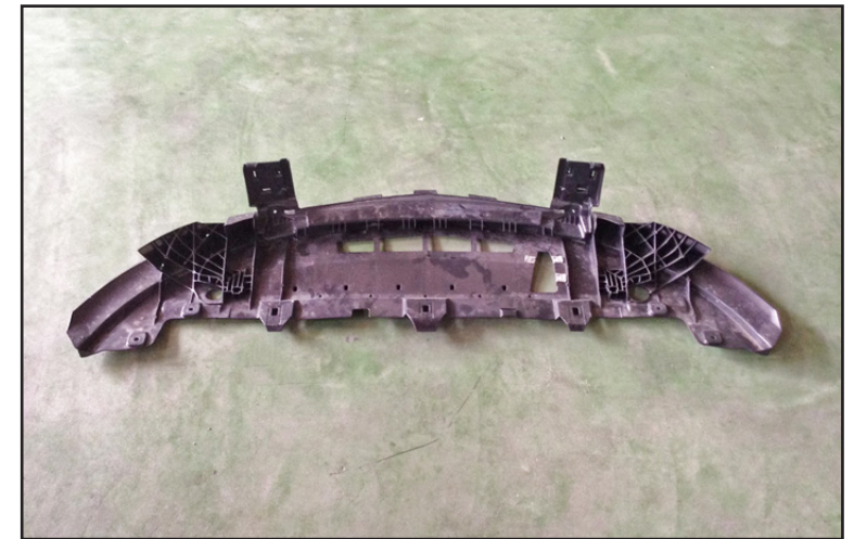
OEM Under Cover. ※Fix OEM under cover to WALD Front Bumper as is on OEM front bumper with the rivets (sold separately).
