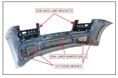
The above picture is Inside of WALD Front Bumper. Need to Cut OEM Parts to replace and fit on WALD Front Bumper.
