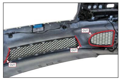
Cut OEM Front Bumper Duct to fit the size of WALD Front Bumper center duct. Cut the attached meshes to fit the both right and left ducts on WALD Front Bumper. Use the attached pins on WALD Front Bumper, then fix them with the caulking glue.
