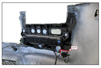
Use caulking glu to fix OEM Head Lamp Brackets on WALD Front Bumper after cutting the corners. \*Cut the corners of OEM Head Lamp Brackets to make the space for PTS.
